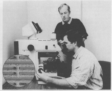
FINE LINES — Bill Bonivert (standing) and John Hachman (at microscope) of Materials Synthesis Dept. 8716 examine micromachine grids manufactured with the LIGA lithography, plating, and molding process. The inset at lower left shows the magnified grid image.
